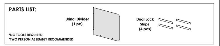
NOTE: Prior to mounting Shield, clean the area where the Dual Lock strips will be applied with a 50/50 mixture of isopropyl alcohol (IPA) and water for proper adhesion.
