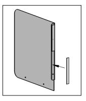
step 4: Take remaining two Dual Lock strips and attach fastener side of each to installed Dual Lock strips on flange of your Divider.
