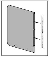
**STEP 5:** Remove the 3M protective film from the two exposed Dual Lock strips. Place Sink Divider up against your desired mounting surface and press down firmly on the flange of Divider. Hold for 30 seconds to ensure proper adhesion of the Dual Lock tape strips to the desired surface and to ensure strips are firmly fastened to each other. **ASSEMBLY COMPLETED**
