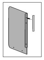
**STEP 3:** Remove the 3M protective film from a second Dual Lock tape strip and apply the adhesive side to rear of vertical flange on Divider, slightly below already installed strip.
