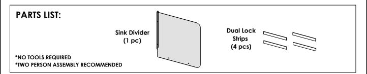
NOTE: Prior to mounting Shield, clean the area where the Dual Lock strips will be applied with a 50/50 mixture of isopropyl alcohol (IPA) and water for proper adhesion.
